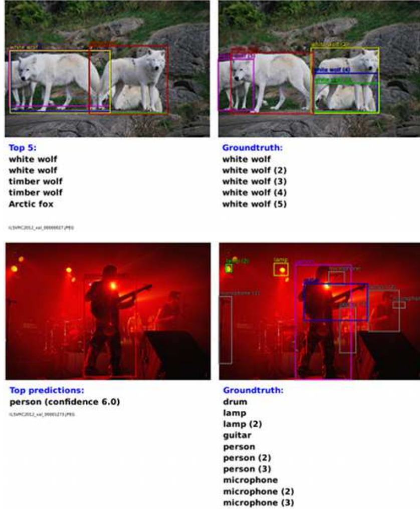
Figure 1: Localization (top) and detection tasks (bottom). The left images contains our predictions (ordered by decreasing confidence) while the right images show the groundtruth labels. The detection image (bottom) illustrates the higher difficulty of the detection dataset, which can contain many small objects while the classification and localization images typically contain a single large object.
